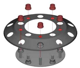
Installation Tip - Our products are designed to install easily, without removing the wheel or all fasteners. Simply remove five (5) of the lug nuts, slip the Wheel Cover over the wheel, and secure with the lug nuts you removed earlier.
