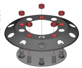
Installation Tip - Our products are designed to install easily, without removing the wheel or all fasteners. Simply remove five (5) of the lug nuts, slip the Wheel Cover over the wheel, and secure with the lug nuts you removed earlier.
